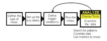
Once you have run a measurement and filled the logic analyzer's acquisition memory with captured data, you can display it with one of the display tools.
