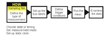
There are two logic analyzer sampling modes to choose from: *timing mode* and *state mode*.
