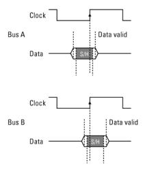
To position the setup/hold window (sampling position) within the data valid window, a logic analyzer has an adjustable delay on each sampling clock input (to position the setup/hold window for all the channels in a pod).
